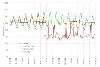
Figure 4: Cooling effect of the system before and after activation of postcooling. Lines indicate temperatures of outdoor air (green), supply air after postcooling (red), extract air (yellow) and setpoint for extract (black).
