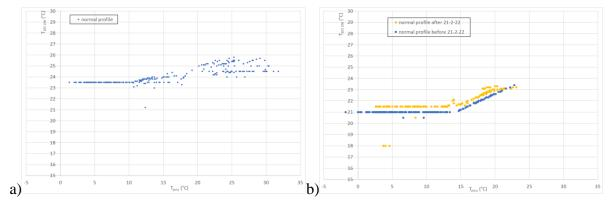
Figure 7: Desired indoor temperature as a function of the prevailing mean ambient temperature  $T_{pma}$  for the house in Italy (a) and in Luxembourg (b). During the course of the year, the residents sometimes change the settings, which - in the case of the house in Luxembourg - has been indicated with blue and yellow dots.
