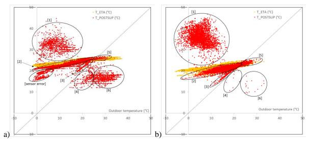
Figure 5: Temperature correlation of supply air (red) and extract air (yellow) as a function of outdoor temperature for the house in Italy (a) and in Luxembourg (b)
