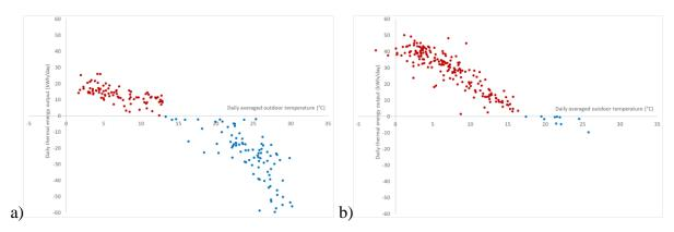
Figure 8: Energy signatures (daily thermal energy output as a function of daily averaged outdoor temperature) for heating in red and for cooling in blue for the house in Italy (a) and in Luxembourg (b).
